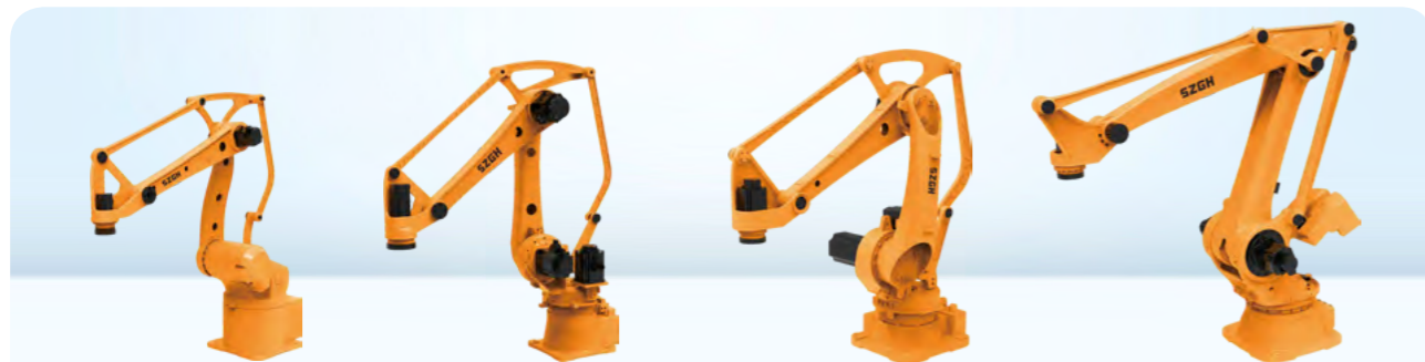
SZGH-B series is a 4-axis robotic arm professionally used in loading and unloading handling and palletizing.
