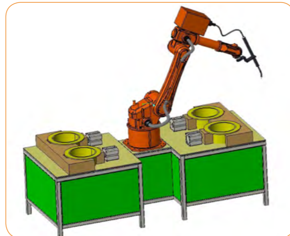
• Application of 4-station welding robot
